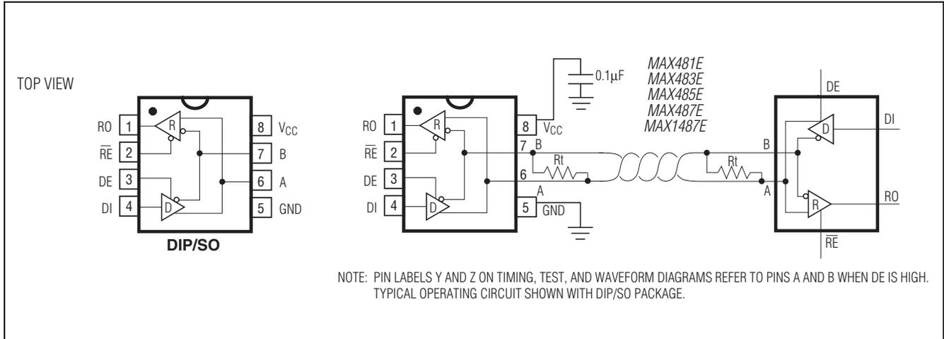
Figure 1. MAX481E/MAX483E/MAX485E/MAX487E/MAX1487E Pin Configuration and Typical Operating Circuit
