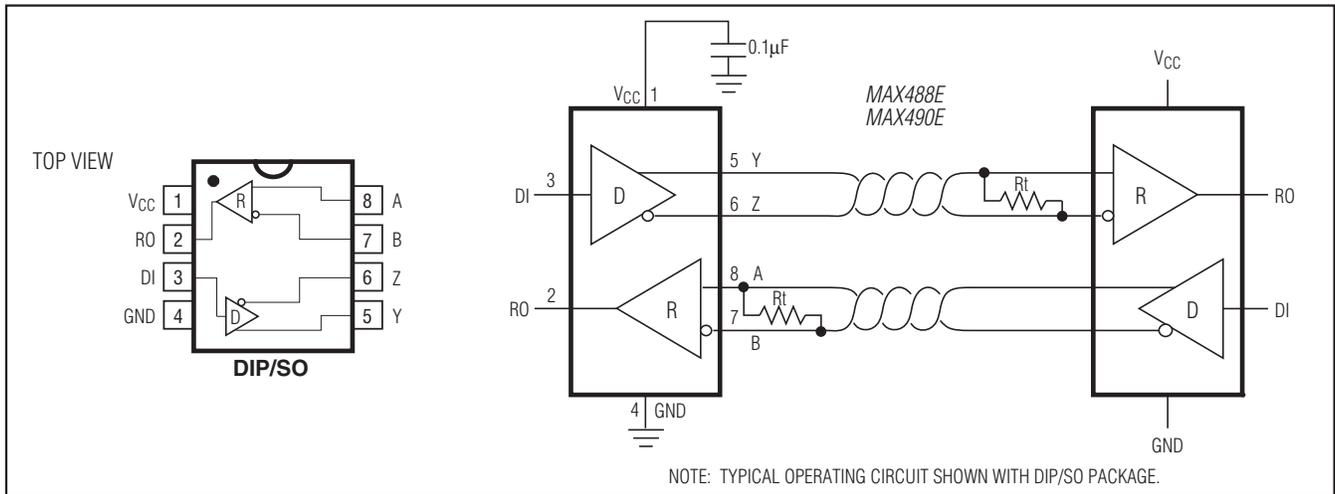
Figure 2. MAX488E/MAX490E Pin Configuration and Typical Operating Circuit
