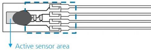
*Area to be covered on the HYT 271 in the assembly for the application in condensing environment*
