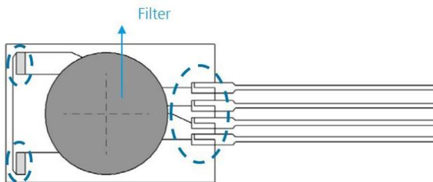
*Area to be covered on the HYT 221 in the assembly for the application in condensing environment*
