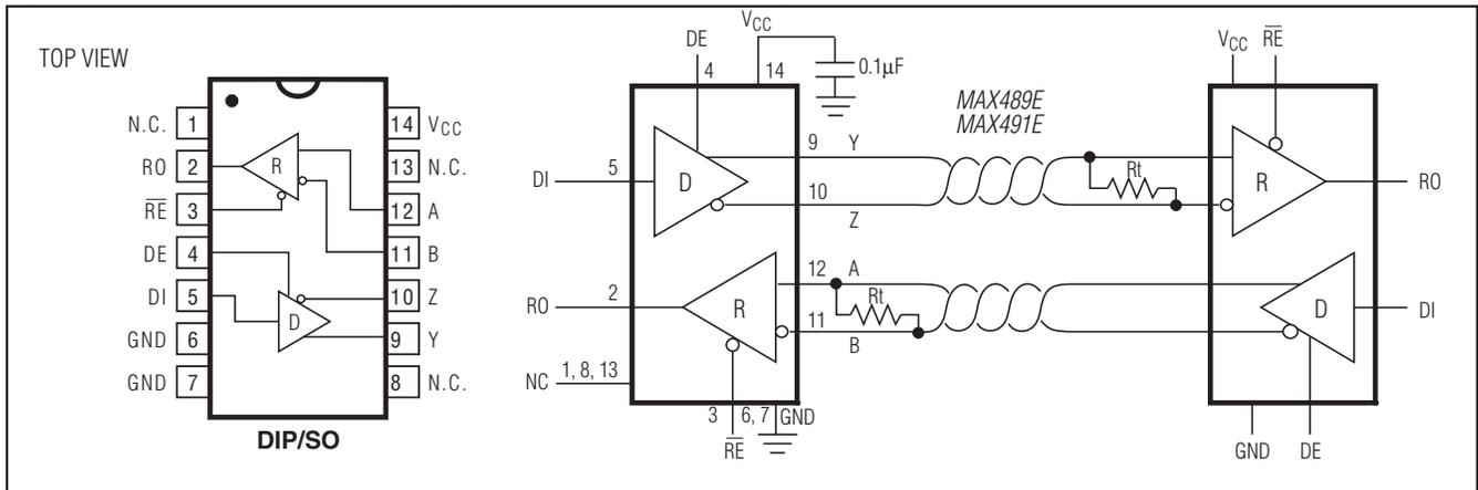
Figure 3. MAX489E/MAX491E Pin Configuration and Typical Operating Circuit
