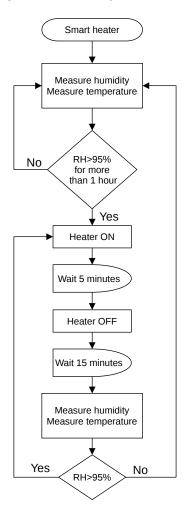
Figure 21: Heater algorithm
