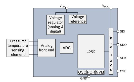
Figure 13: Pressure sensor: block diagram
