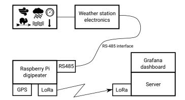
Figure 22: Block diagram of the prototype
