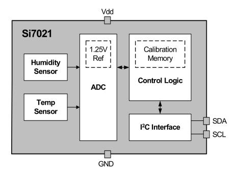
Figure 11: Humidity sensor: block diagram
