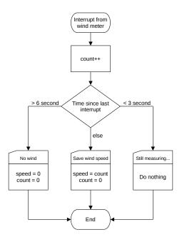
Figure 19: Wind speed interrupt
