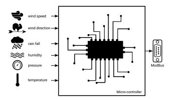
Figure 3: Block diagram of weather station
