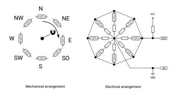
Figure 7: Wind vane: theory of operation
