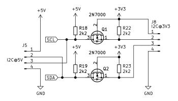
Figure 15: I<sup>2</sup>C bus level shifter
