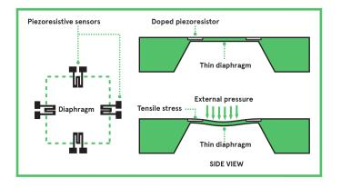
Figure 12: Piezo-resistive pressure sensor
