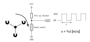
Figure 5: Cup anemometer: theory of operation
