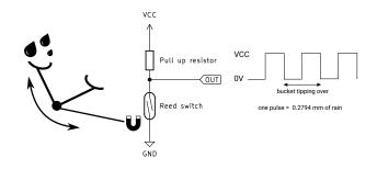
Figure 9: Rain meter: theory of operation
